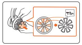
NOTE: There are cases in which some fixing claws are not fixed properly even if the wheel cover is assembled. Please press the wheel cover to make sure that all the fixing claws are in place.
