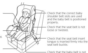
twisted or loose. Always pull down the baby waist example of use in child mode belt to firmly hold the pelvis position.
