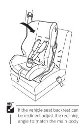
① Slowly pull out the seat belt making sure that it is not twisted. 2 Route the seat belt through the seat belt guide
