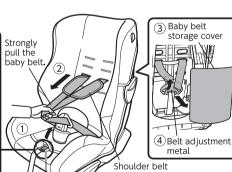
belts from the storage cover from the back of the main shoulder belt body. 4 Unhook the left and right baby belts from the belt adjustment metal.
