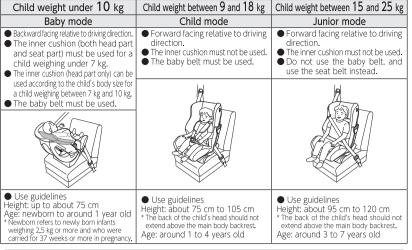
Always use backward facing mode for children weighing under 9 kg. Do not use forward facing mode in this case, as this is extremely dangerous to the child.
