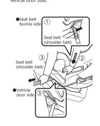
With the seat belt (shoulder belt) strongly pulled, route the seat belt shoulder belt) under the side wall and clasp it with the belt guide ® on the vehicle door side.
