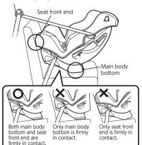
Use the "Angle Checker" on the front side of this user manual as a guide when installing the child car seat in backward facing mode
