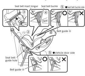
Mhile pressing the main body against the vehicle seat, pull the seat belt (shoulder belt) to remove any looseness in the seat belt (waist belt).
