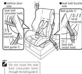
1) Place your knee deeply into the seat and apply body weight to press the main body down onto the vehicle seat.
