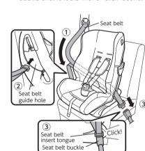
1 Route the seat belt (waist belt) through the left and right belt guides ©. ② Route the seat belt (shoulder belt) through the belt guide ©
