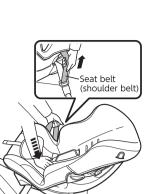
Route the seat belt (shoulder belt) through the belt guide (A) on the seat belt buckle side 2) Press the main body against the vehicle seat
