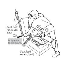
3 With the seat belt (shoulder belt) strongly pulled, open the red locking device on the vehicle door side. 4 Insert the seat belt (shoulder belt) to the top of the open locking device, and press the locking device to
