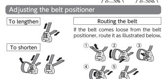
The belt positioner should be adjusted so that the seat bel noulder belt) holds the child's shoulder at the correct position • WARNING Adjust the height as the child grows and the belt positions
