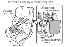
4 Pull out the left and right shoulder belt covers one at a time from the back of the main body. ⑤ Release the left and right guide clip slots on the upper part of the seat cover from the guide clips, unhook the left and right attachment loops and the hooks, and remove the seat cover.
