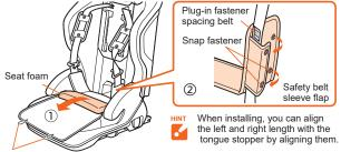
Fixing rubber band for seat cloth sleeve
