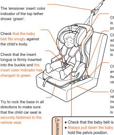
Check that the baby belt is adjusted to the correct position.
