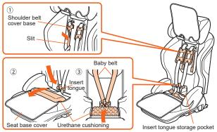
① Attach the right and left seat base cover installing rubber rings. 2 Attach the right and left head guard cover installing rubber rings.
