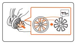
NOTE: There are cases in which some fixing claws are not fixed properly even if the wheel cover is assembled. Please press the wheel cover to make sure that all the fixing claws are in place.
